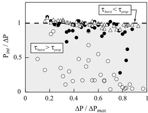
**Figure 2.** Normalized amplitude  $P_{int}/\Delta P$  of the acoustic signal at bursting, inside the cavity, as a function of the initial normalized overpressure  $\Delta P/\Delta P_{max}$ .  $P_{int}/\Delta P < 1$  (gray region) indicates a slow dynamics of the film opening. [Symbol,  $\alpha$ ]: [ $\circ$ , 2]; [ $\bullet$ , 8]; [ $\triangle$ , 23].
