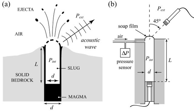
**Figure 1.** (a) Sketch of a slug exploding at the top of a volcanic conduit. (b) Experimental setup of a soap film bursting at the surface of a cavity of well controlled geometry (length  $L$ , diameter  $d$ , volume  $V$ ) and initial overpressure ( $\Delta P$ ).
