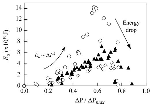
**Figure 4.** Acoustic energy  $E_a$  as a function of the initial overpressure  $\Delta P$  (normalized to  $\Delta P_{\max}$ ) for different lengths (same diameter  $d = 8$  mm). All data represent the maximum pressure recorded outside over a series of ten measurements. We assume that this value corresponds to the signal recorded when the rupture time is negligible ( $\tau_{burst}/\tau_{prop} < 1$ ). [Symbol,  $\alpha$ ]: [ $\circ$ , 2.5]; [ $\blacktriangle$ , 5]; [ $\diamond$ , 6.9].
